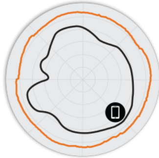
Figure 3. R750 5GHz AzimuthAntenna Patterns
