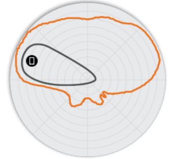
Figure 5. R750 5GHz Elevation Antenna Patterns
