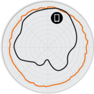
Figure 2. R750 2.4GHz AzimuthAntenna Patterns
