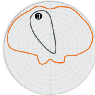
Figure 4. R750 2.4GHz Elevation Antenna Patterns
